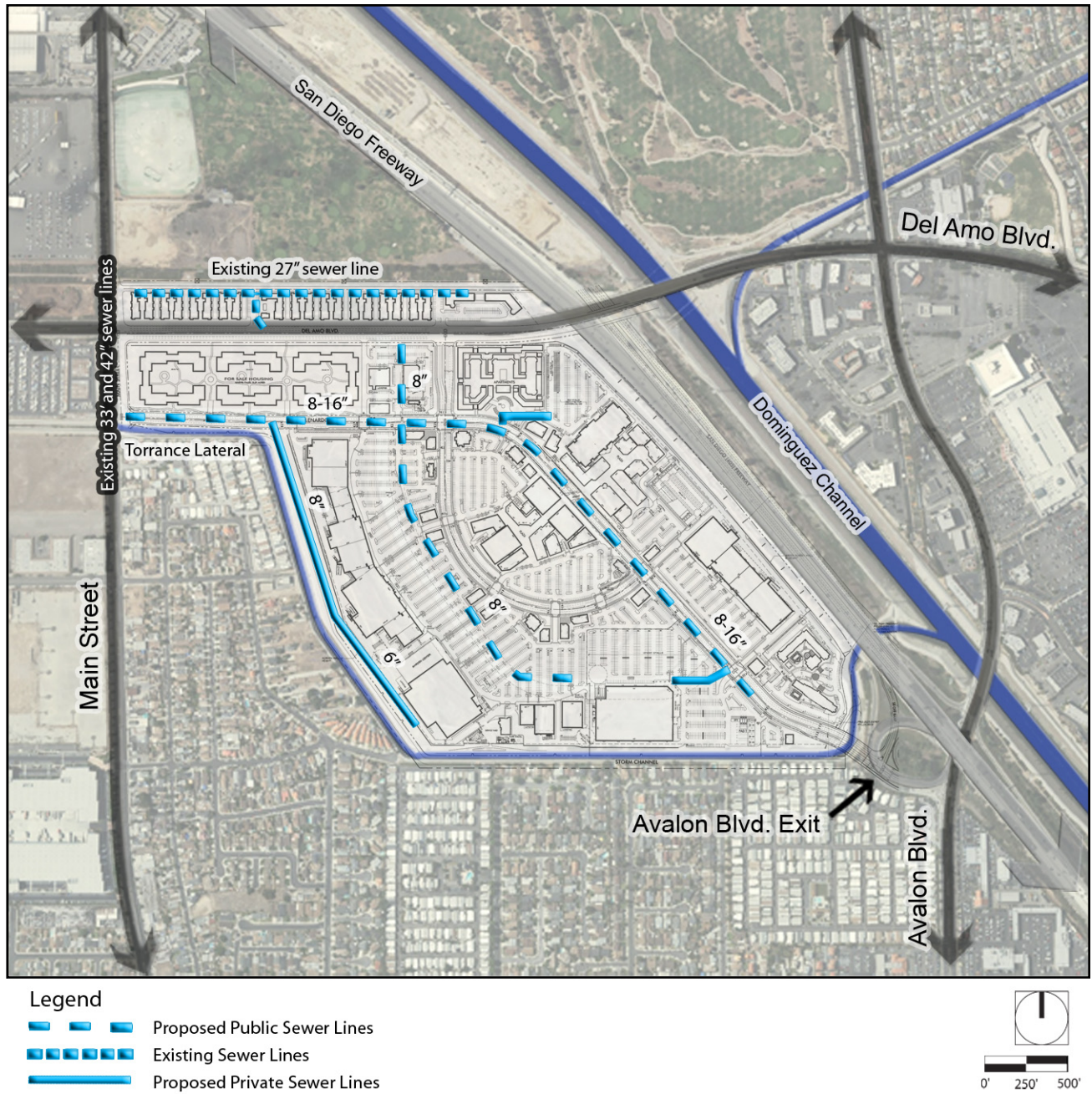
Figure 5.4b Sanitary Sewer Concept
